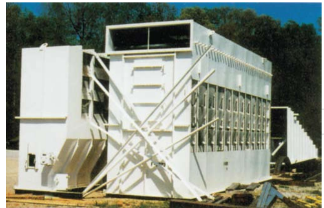
ACT Continuous fluid bed/baghouse combination, unassembled and ready for shipment. Left to right: Fluid bed, baghouse top and air plenum (In background).
