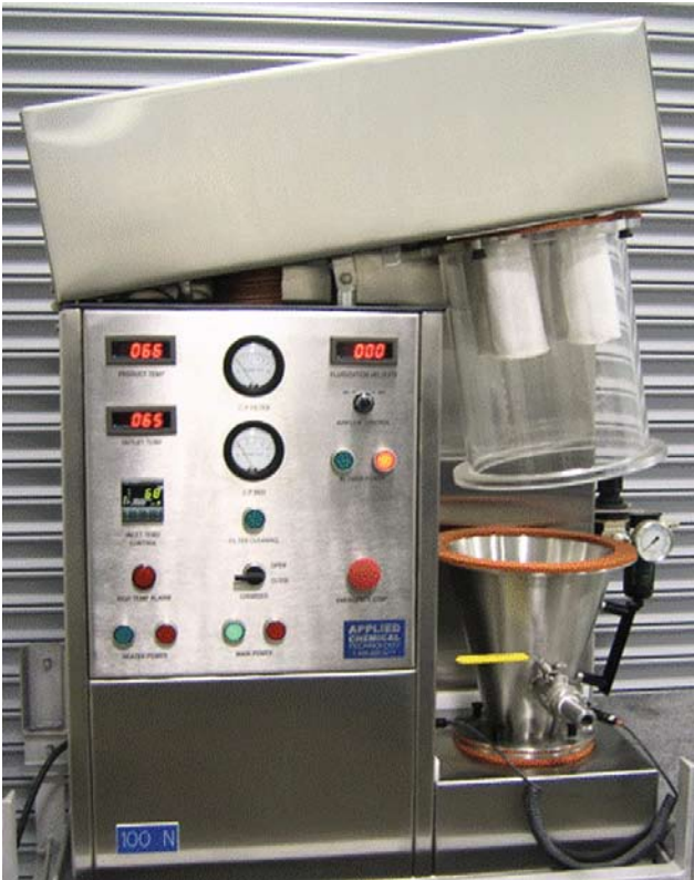
ACT Laboratory Fluid Bed Dryer/ Granulator/Coater - Model 100N. Standard model includes batch operation, variable speed blower, full pressure and temperature instrumentation, air temperature up to 250°F.
