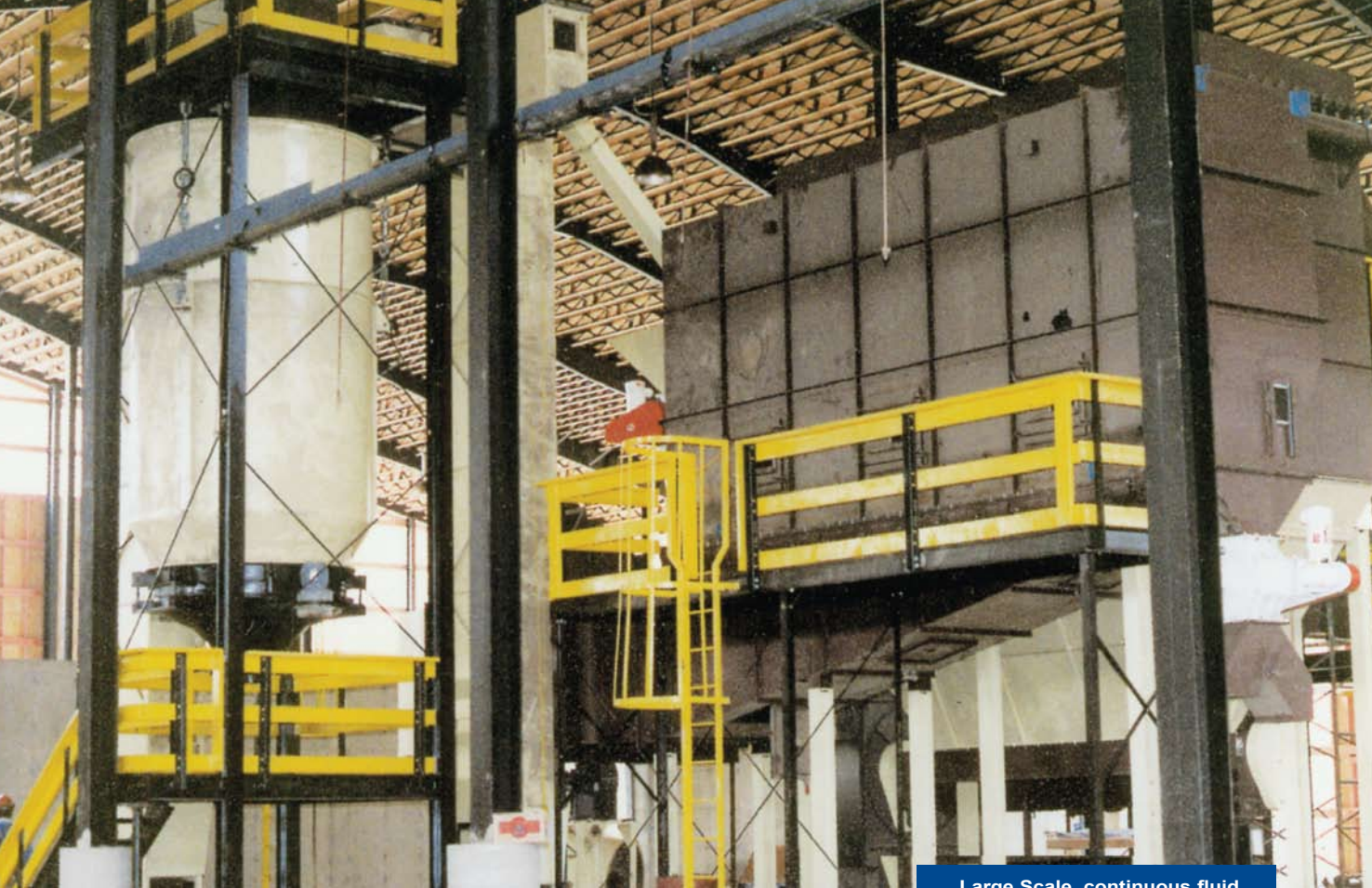
Large Scale, continuous fluid bed/baghouse combination, installed in production plant.
