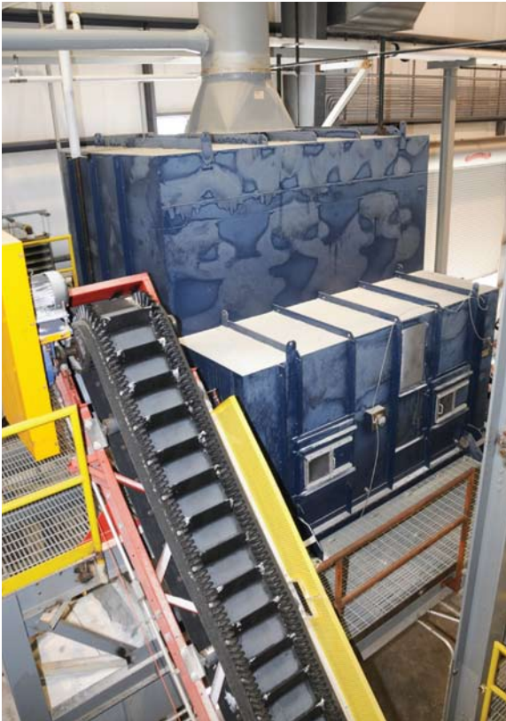
Fluid bed/baghouse cooler for continuous operation.
